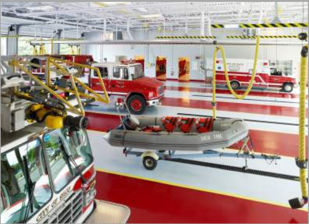
Apparatus Bays: The five drive-through apparatus bays include a radiant heated slab with 14' x 14' doors that will accommodate the largest of ladder trucks.
