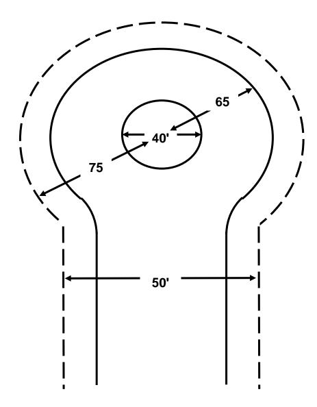
UTILITIES ARE PROHIBITED FROM BEING INSTALLED IN THE CENTER OF THE CUL-DE-SAC IF ALTERNATIVE INSTALLATION CAN BE PROVIDED
