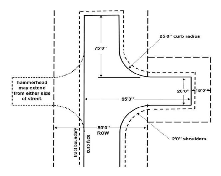
Dimensions shown are from curb face to curb face. The total size of the street tract will vary, to accommodate setbacks, sidewalks, street trees, stormwater facilities, and any other right of way elements.
