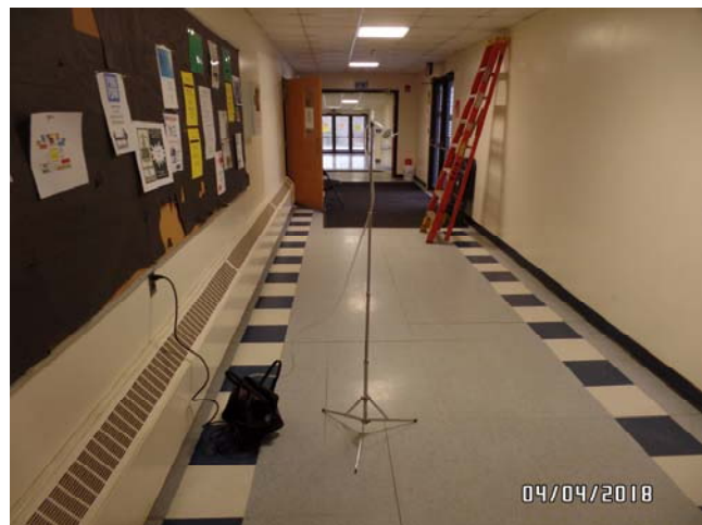
Mold Air Sample (A-4) in corridor near Multi Purpose Room.
