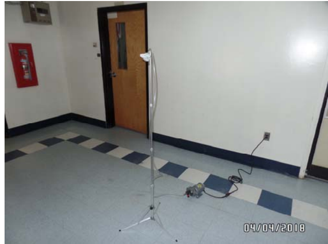
Mold Air Sample (A-8) in corridor near Room #22.
