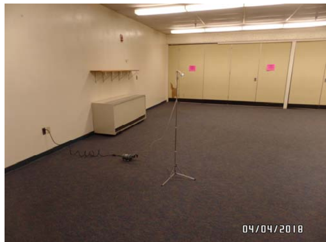
Mold Air Sample (A-6) in Room #26.
