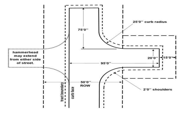
Dimensions shown are from curb face to curb face. The total size of the street tract will vary, to accommodate setbacks, sidewalks, street trees, stormwater facilities, and any other right of way elements.
